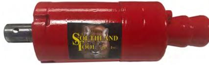
**RED HOT** The round profile of the cutters allows it to enter sewer lines from 4" and up. The motor can accommodate hose sizes of 1" and 3/4" with flow from 35 to 80 gpm and pressure from 2000 to 3000 psi. Rated up to maximum of 235 lbs. of torque and 175 lbs. at continuous operation. This tool has the power to clean while the bearing can take a beating and keep on ticking. This motor beat all competitor motors.
