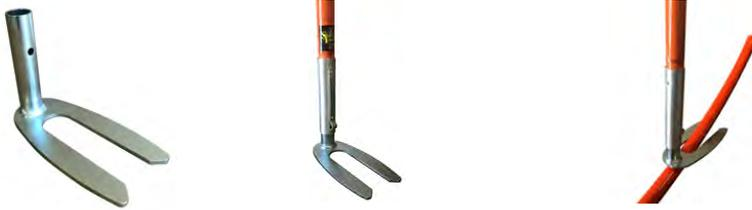
**SHT-1** 7" WIDE OPPOSITE HOSE GRABBER, OPPOSING C HOOKS GRAB HOSE IN MIDDLE AND TWIST FOR EASY GRABBING. ALLOWS YOU TO MOVE THE HOSE FROM SIDE TO SIDE OR PUSH ON IT IN ANY DIRECTION. MADE OF STRONG ¾" SPRING STEEL, ZINC PLATED.
