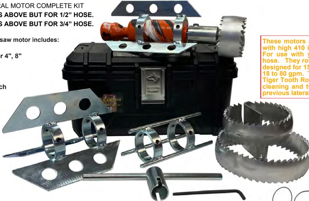
These motors are new and improved with high 410 inch pounds of torque. For use with your 1/2", 3/4" and 1" hose. They rotate at 400 rpm and are designed for 1500 to 400 psi and from 18 to 80 gpm. This new and improved Tiger Tooth Root Cutter has twice the cleaning and twice the power of our previous lateral motors.
