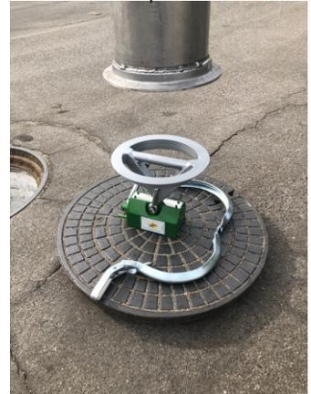
Just place on cover and lower boom to connect. Clamp-up!
